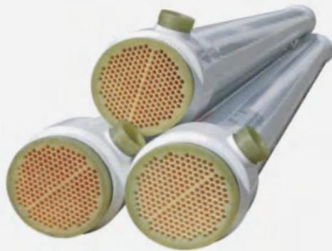
CONSEPTEC TMBR tubular UF membrane is a new type of solid-liquid separation membrane. It is made of PVDF membrane material, the molar weight cut-off(MWCO) ranges from 5kDa to 250kDa. Its high strength, anti pollution and chemical (acid and alkali) resistance makes it widely used in engineering systems.
