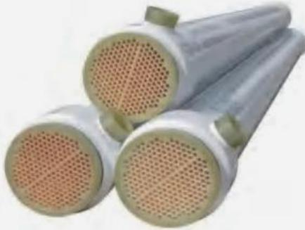
CONSEPTEC TUF membrane is one of the advanced industrial istewater membranes. It is made of PES membrane material, which can withstand the istewater with pH range 2-13, and the molar weight cut-off(MWCO) is generally 100kda. It is widely used in RO concentrated water, cooling circulating water and other high salt water softening processes.
