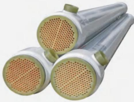
CONSEPTEC TMBR tubular UF membrane is a new type of solid-liquid separation membrane. It is made of PVDF membrane material, the molar weight cut-off(MWCO) ranges from 5kDa to 250kDa. Its high strength, anti pollution and chemical (acid and alkali) resistance makes it widely used in engineering systems.
